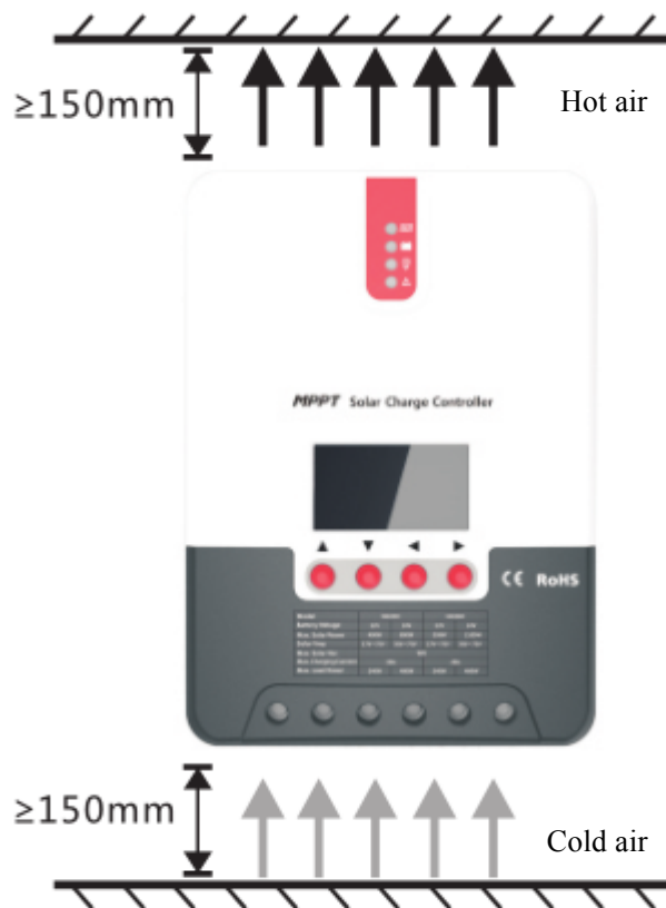
Fig. 2.1 Installation and heat dissipation
